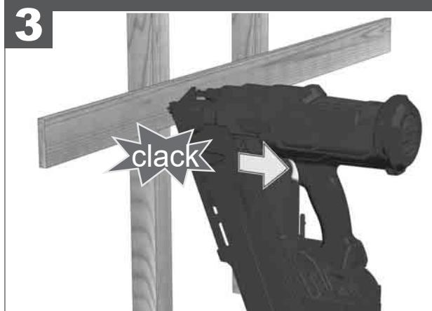
**Switch to single sequential actuation:**
