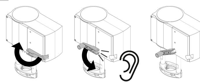
Depending on temperature – in case of high temperature – use instruction for 1-0152285 before mounting actuator! **1.6** Mount the actuator according to step 1-2.3 of the installation instruction for the actuator. Do not yet power up the actuator!
