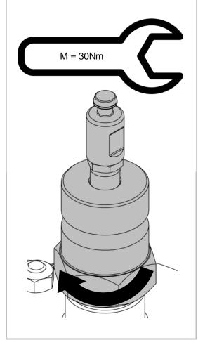
Place the adaptor spindle inside the adaptor nut, then screw the small nut on 1.2 the adaptor spindle as far as it can go, and lastly screw the adaptor top on the adaptor spindle as far as it can go.
