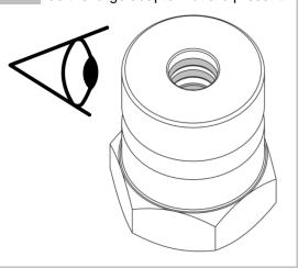
Screw the adaptor nut onto the valve, use a 36mm spanner to tighten it with a torque of 30Nm. Then press until the adaptor spindle has made contact with the top of the
