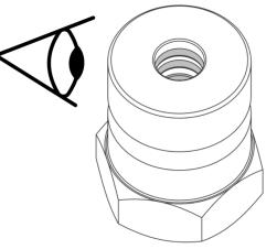
Screw the adaptor nut onto the valve, use a 36mm spanner to tighten it with a torque of 30Nm. Then press until the adaptor spindle has made contact with the top of the valve spindle.
