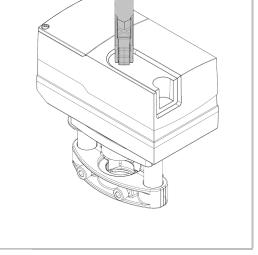
Depending on temperature – in case of high temperature – use instruction for 1-0152285 before mounting actuator! **1.6** Mount the actuator according to step 1-2.3 of the installation instruction for the actuator. Do not yet power up the actuator!
