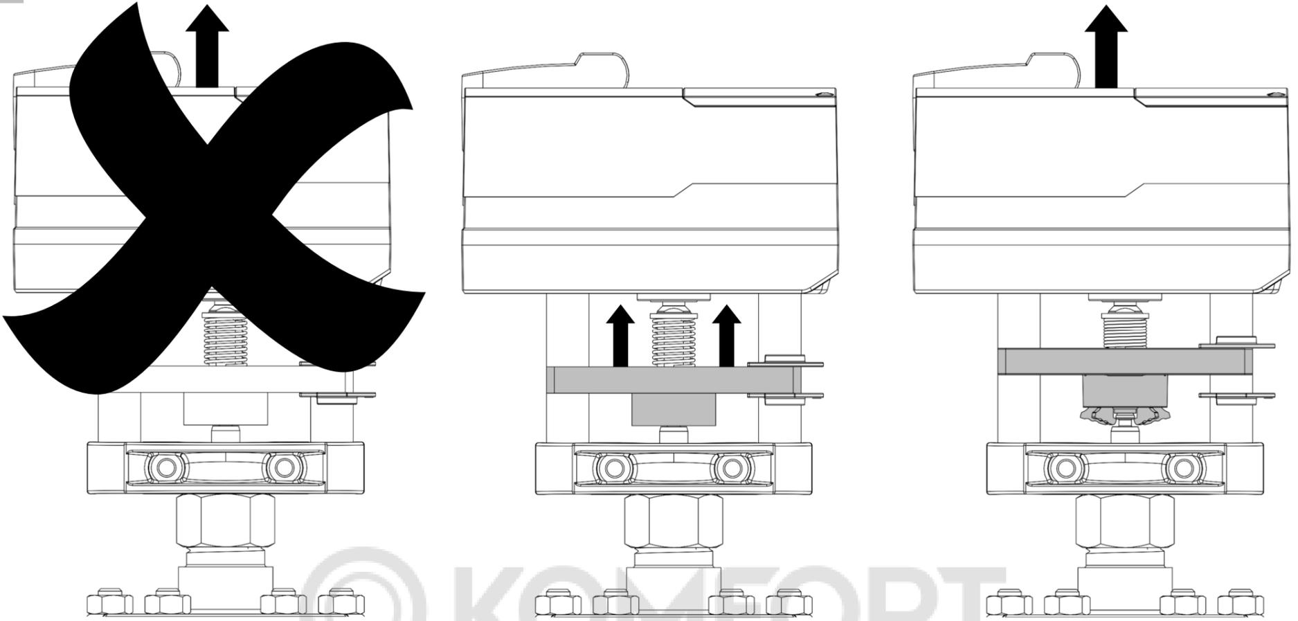
3.1 Before demounting the adaptor, it is important to firstly close-off the inlet and secondly the outlet to the valve!!!
