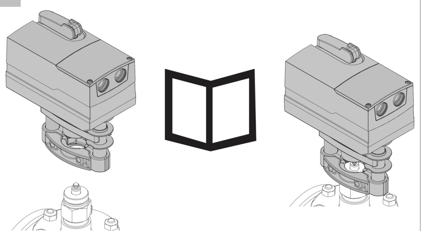
2.1 Before demounting the actuator, please release the actuator's grip on the adaptor spindle!
