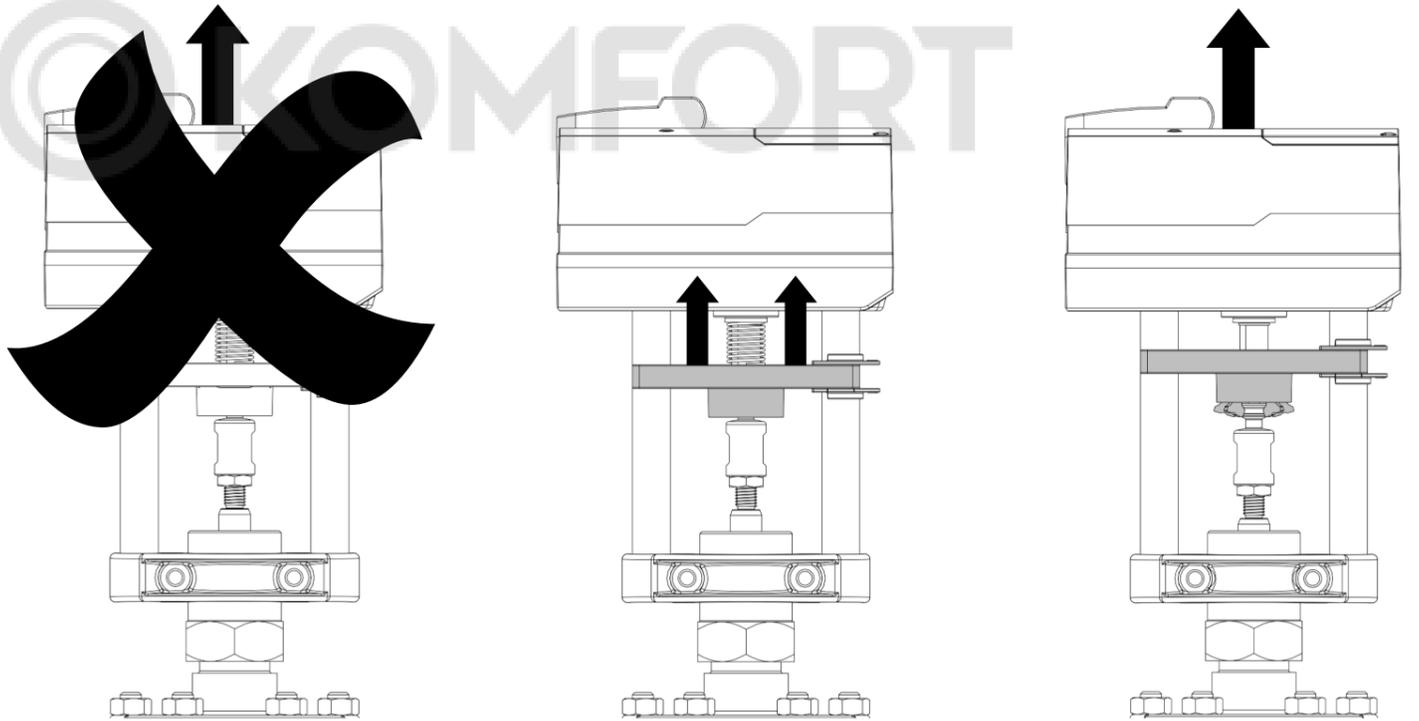
**3.1** Before demounting the adaptor, it is important to firstly close-off the inlet and secondly the outlet to the valve!!!
