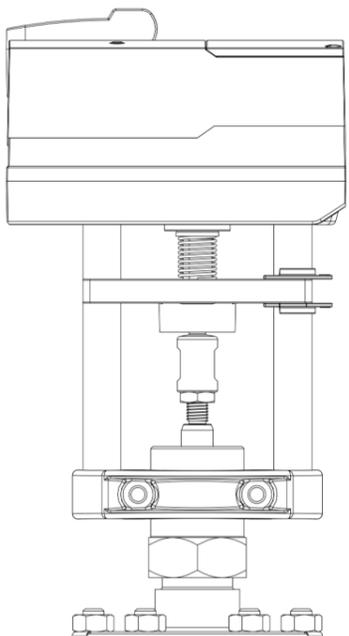
**2.1** Before demounting the actuator, please release the actuator's grip on the adaptor spindle!
